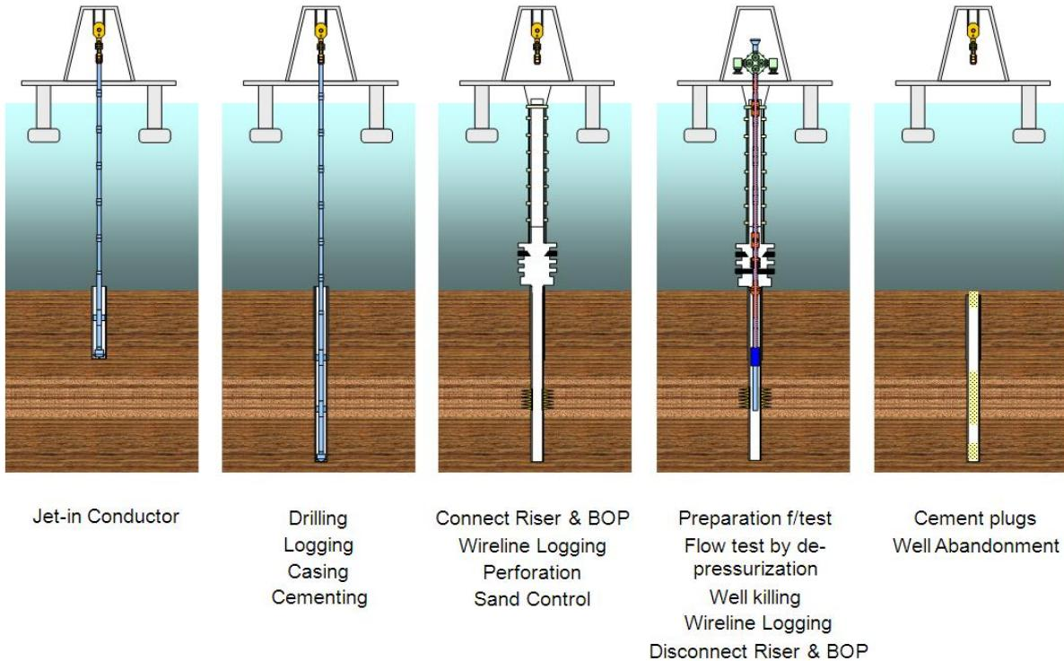
**Figure 7:** Schematic of proposed marine production test design planned for 2012-2013 in the Nankai Trough (from *Masuda et al., 2010a*).
