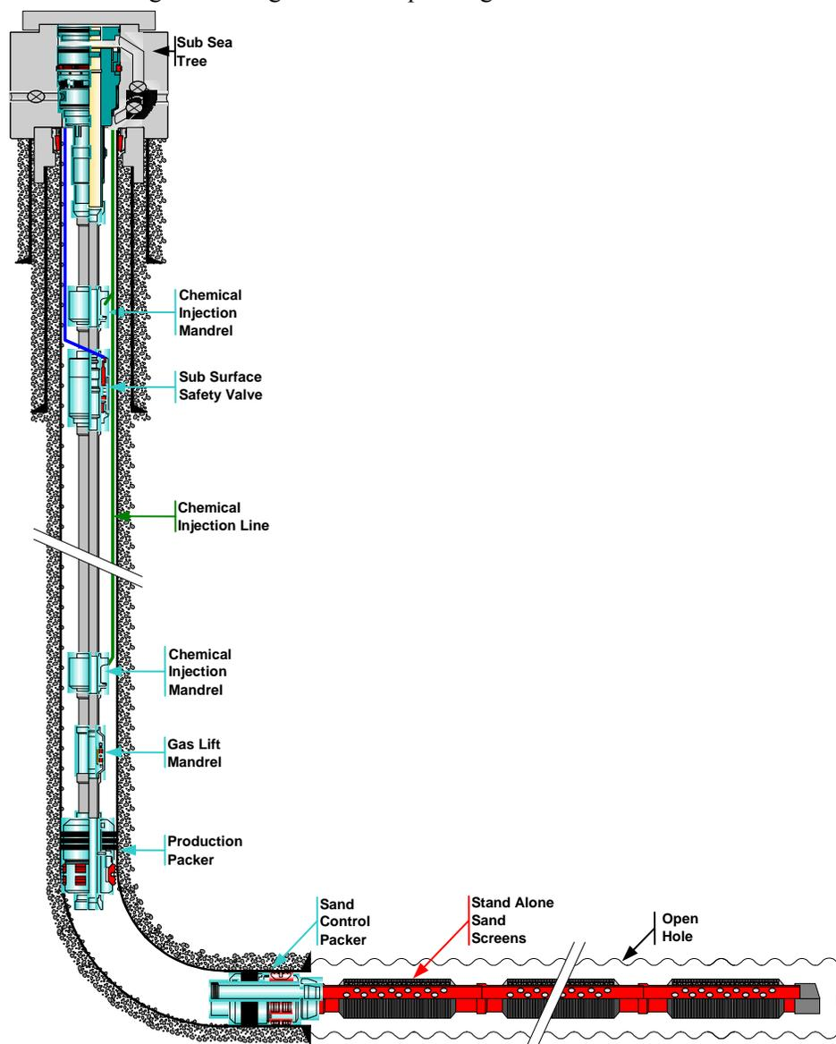
**Figure 6:** Schematic well design for deepwater marine gas hydrate production (from *Hancock et al., 2010*; ©2011, Offshore Technology Conference).
