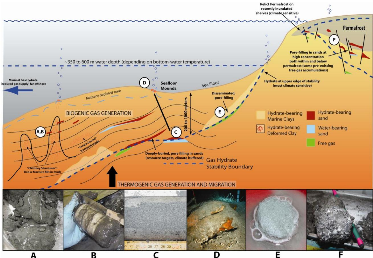
**Figure 1:** Geologic environments of gas hydrate occurrence. Photos of gas hydrate morphologies observed in nature are shown along bottom courtesy of: A) UBGH-01 Science Party; B) NGHP-01 Science Party; C) JOGMEC; D) Ian MacDonald; E) GMGS-01 Science Party; F) JOGMEC, NRCan, USGS.
