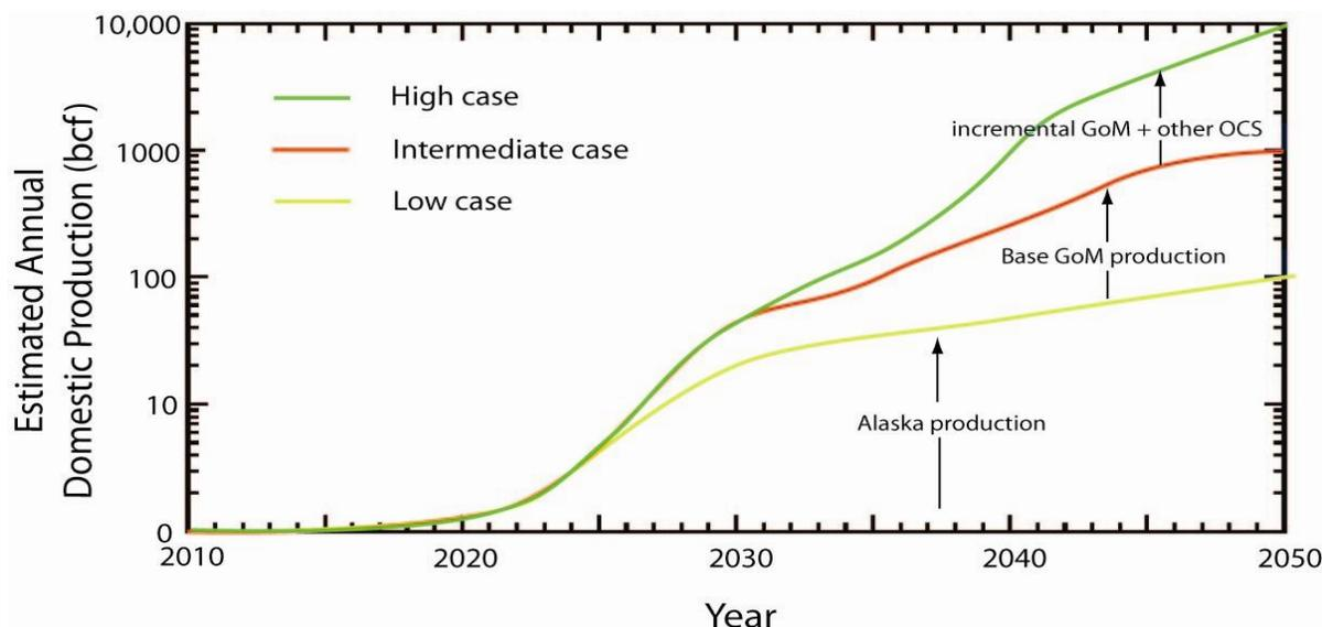
**Figure 8:** Speculative schematic of three potential annual domestic production scenarios for gas hydrate resources through 2050. Scenarios explained in the text.
