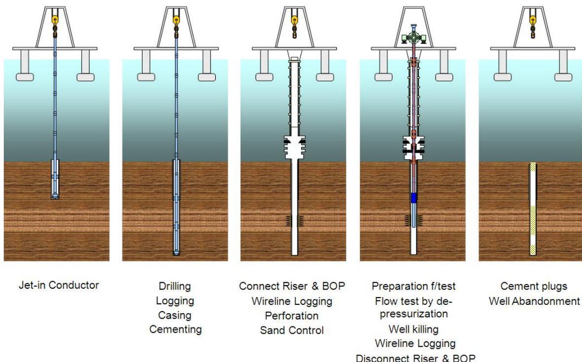
**Figure 7:** Schematic of proposed marine production test design planned for 2012-2013 in the Nankai Trough (from *Masuda et al., 2010a*).
