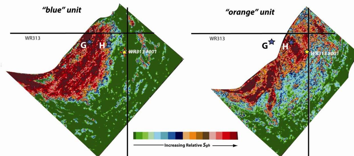
**Figure 4:** Pre-drill predictions of gas hydrate saturation within reservoir units in Walker Ridge block 313, northern Gulf of Mexico (modified from *Shelander et al., 2010*; also as used by permission of OTC). LWD data for the reservoir shown on the right at the well location “H” shown in Figure 2.
