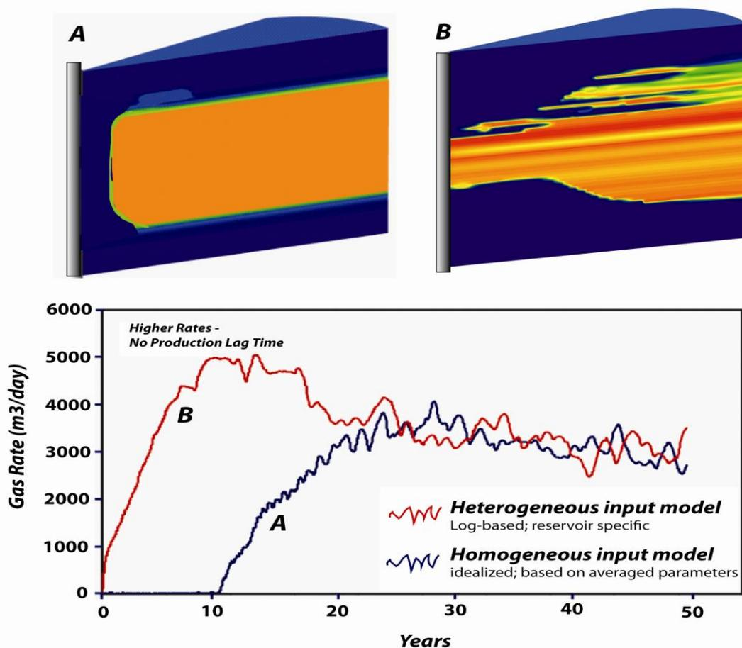
**Figure 5:** Comparison of modeled production response between homogeneous (A) and heterogeneous (B) reservoir models based on data from the Mount Elbert test well in Alaska. The consideration of vertical heterogeneities results in high production volumes and reduced or eliminated production lag times (modified from Anderson *et al.*, 2011b).
