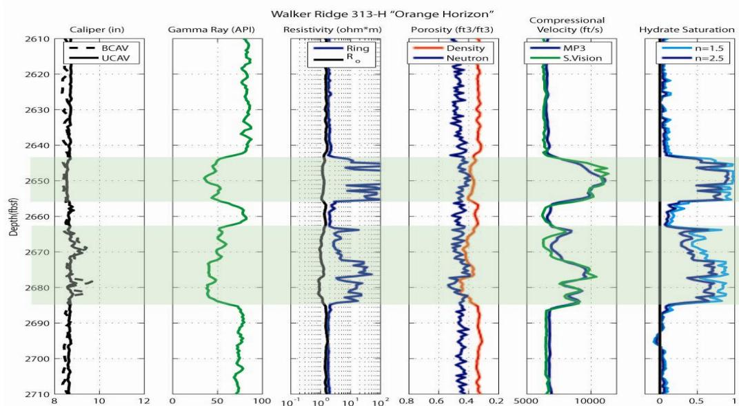
**Figure 2:** Logging-while-drilling data for gas hydrate-bearing sand in Walker Ridge block 313. Light green interval is the hydrate-bearing section (from *Boswell et al., 2010*, courtesy OTC).
