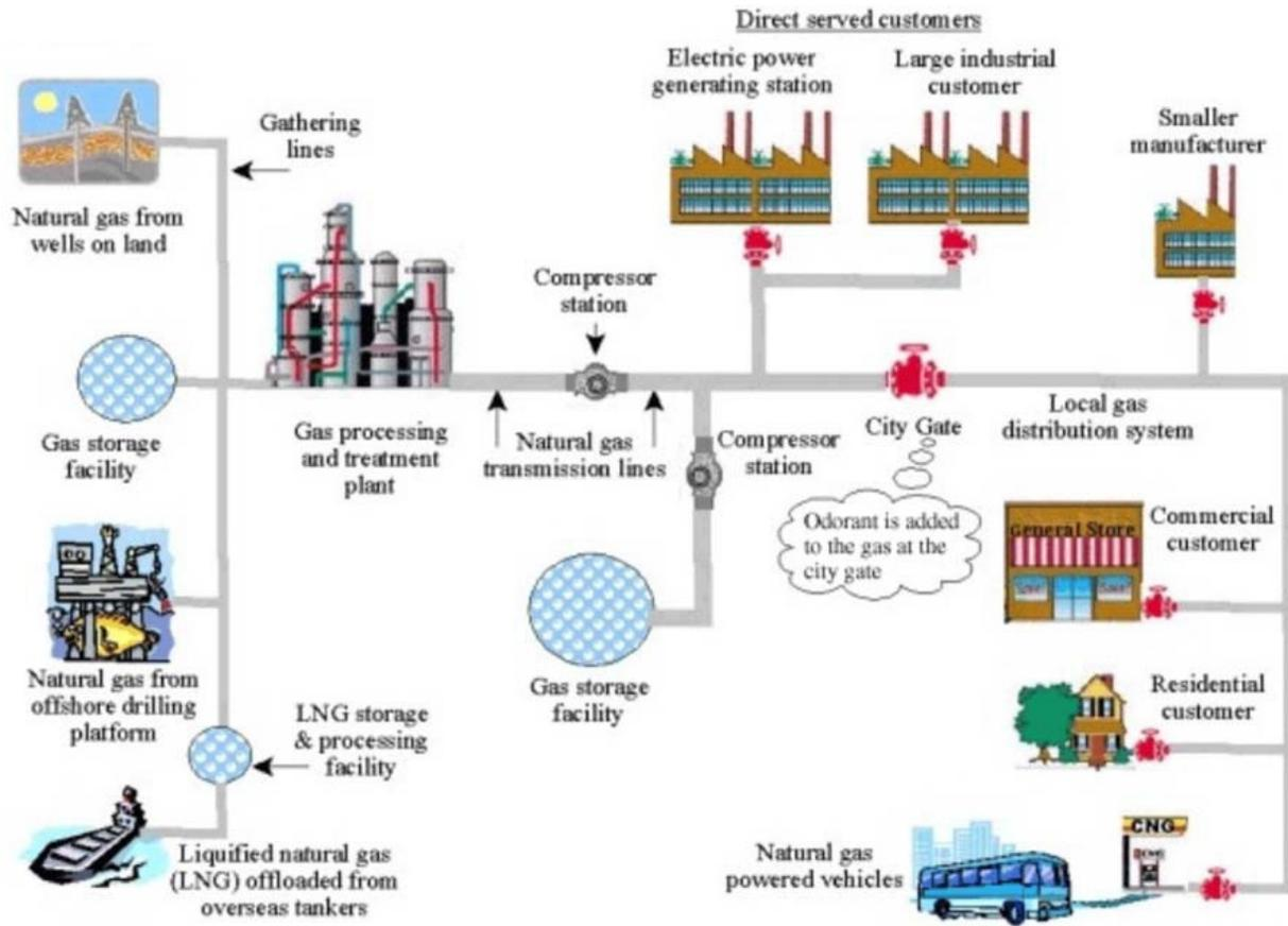
Figure 1. Schematic of a Typical Natural Gas Pipeline System (PHMSA, 2010a)
