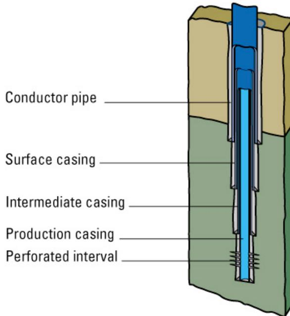
Figure 3. Types of casing.
