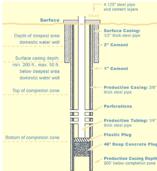
Figure 2. Example of a gas well (diagram is not to scale and has been dramatically shortened).<sup>35</sup>
