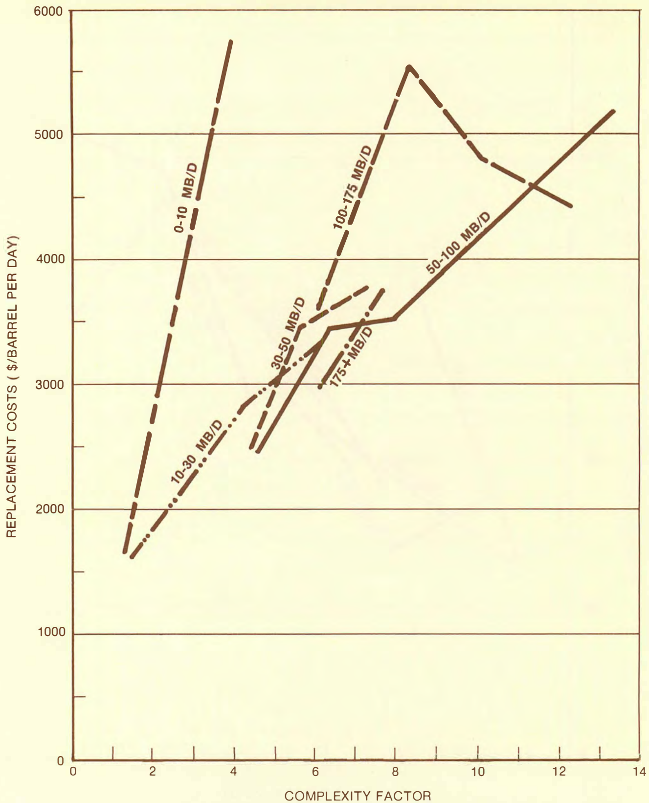
Figure 48. 1978 Replacement Costs as a Function of Complexity— Aggregated by Refinery Size Range.
