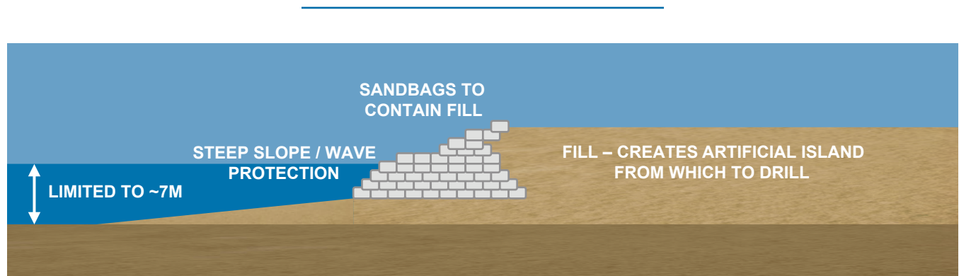
Figure 1-18. Typical Sandbag Retained Island Schematic
