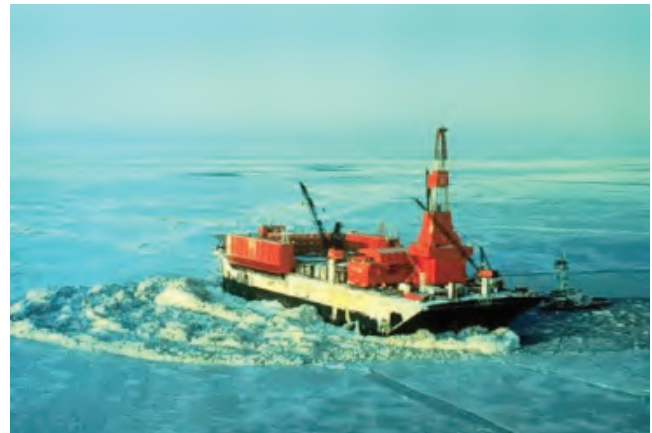
Figure 1-32. The SSDC/MAT—Now Known as the SDC (Steel Drilling Caisson)
