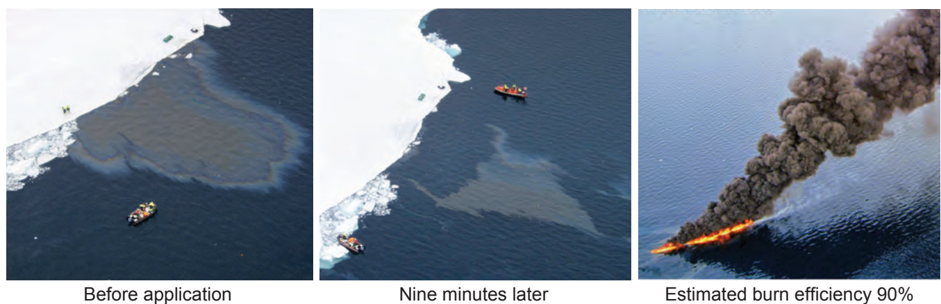
Figure 8-16. Photo Sequence Showing Before and After Shots During the First Field Test of Herders under Arctic Conditions in Norway, 2008
