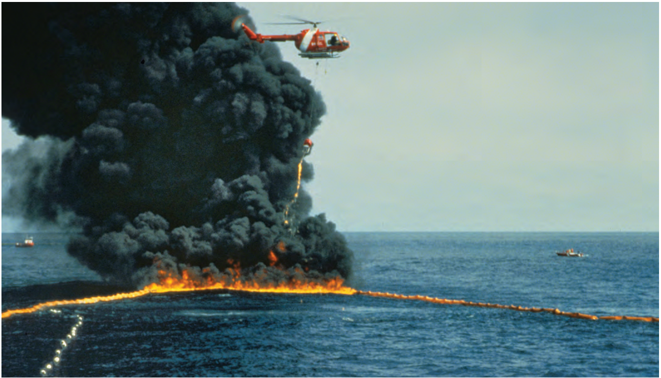
Figure 8-13. Open Water Burning of Crude Oil in a Fireproof Boom after Ignition with a Helitorch™ During the Newfoundland Offshore Burn Experiment in 1993
